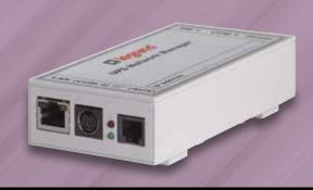
They are special network devices designed to autonomously manage UPS. External software is not required: a 32-bit processor resides in the board along with an operating system of the "UNIX Embedded" type which is able to continuously monitor the operation of the UPS, handle lots of events (power failure, overload, bypass, faults,...).
