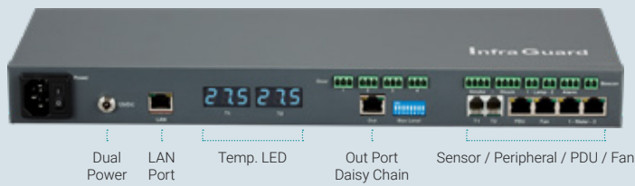
EC-300M - Master Control Box (1st Level)
