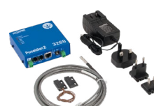
Poseidon2 3268 TSet includes a temperature sensor, door contact and a power adaptor.
