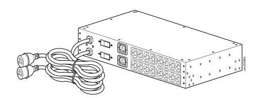
**Input power cords:** The two cords connect the ATS to two separate power sources (A, B). The switch draws power from the preferred source and automatically switches to the secondary source when necessary. The two (2) 2.44-m (8-ft) power cords have IEC-309 32 A plugs.
