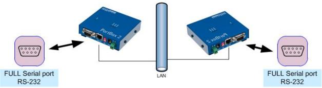
Serial port extension. The serial port is configured for 19000 Bd, 8N1, SW handshake.
