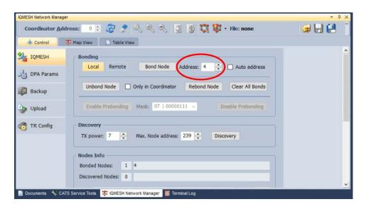
3. In the IQMESH Network Manager, go to the Control tab, and enter address 4 in the IQMESH menu.
