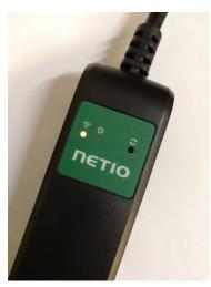
6. After a successful bonding, a message about the bonding result appears and the yellow LED lights up on the PowerCable IQRF.
